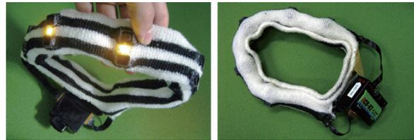
Fig. 3. The TR with its washable protective tissue, also showing the LED indicators (one per module). (Colours are visible in the online version of the article; <http://dx.doi.org/10.3233/TAD-140414>)
