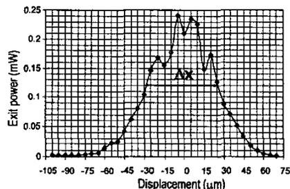
Figure 6 Alignment tolerance for a channel
