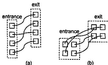
Figure 3 Basic interconnection used in the Banyan example
